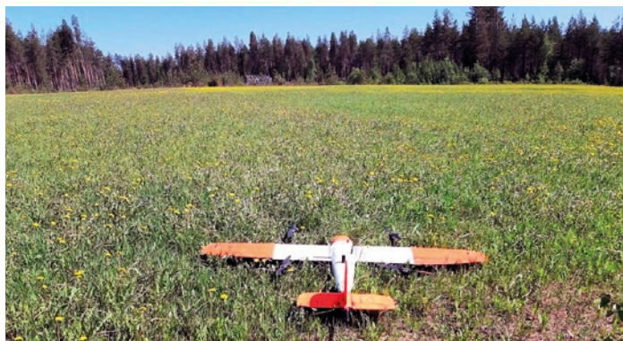
UAV ready for a take-off for Anomaly 5 magnetic survey.
