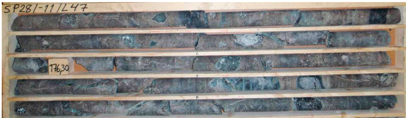
Core from recent drilling at Seitaperä showing mantle xenoliths
